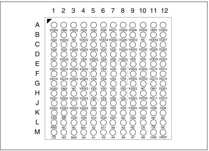
Note: Vss balls inside the dotted box are optional for purposes of thermal dissipation.
