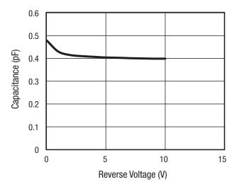
Figure 1. Total Capacitance vs Reverse Voltage
