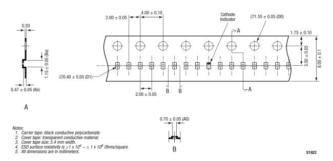
Figure 3. SOD-882 Tape and Reel Dimensions
