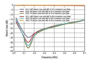
Figure 7. Return Loss vs Frequency (ANT, TX, and RX Ports; Vctl = 28 V, Ictl = -50 mA)
