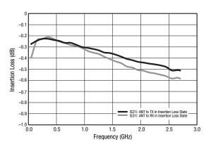
Figure 10. Insertion Loss vs Frequency (ANT to RX and ANT to TX Ports; VctL = 5 V, IctL = -50 mA)
