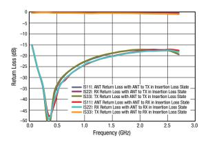
Figure 14. Return Loss vs Frequency (ANT, TX, and RX Ports; Vctl = 5 V, Ictl = -50 mA)
