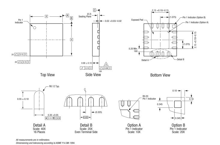
Coplanarity applies to the exposed heat sink slug as well as the terminals.
