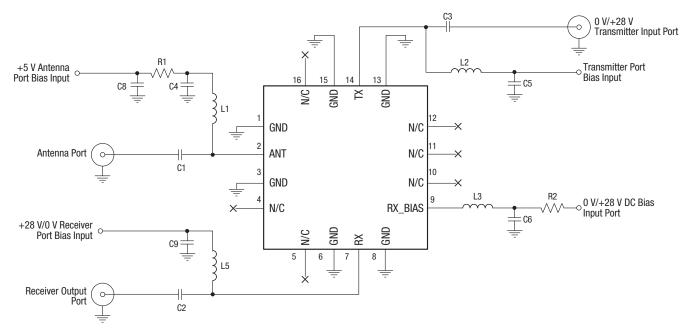
NOTE: The N/C pins (4, 5, 10, 11, 12, and 16) are not internally connected, so they can be left open or grounded.
