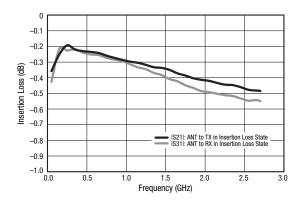
Figure 9. Insertion Loss vs Frequency (ANT to RX and ANT to TX Ports; Vctl = 28 V, Ictl = -50 mA)
