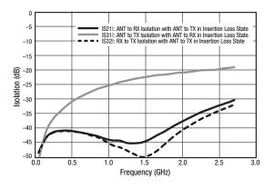
Figure 12. Isolation vs Frequency (ANT to RX, TX to RX, and ANT to TX Ports; VCTL = 5 V, ICTL = -50 mA)
