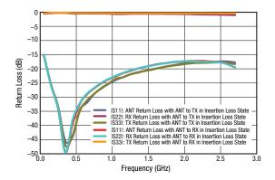
Figure 13. Return Loss vs Frequency (ANT. TX. and RX Ports: Vct. = 28 V. lct. = -50 mA)
