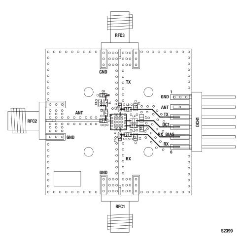
Figure 22. SKY12208-306LF Evaluation Board Assembly Diagram
