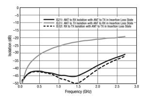
Figure 11. Isolation vs Frequency (ANT to RX, TX to RX, and ANT to TX Ports; VctL = 28 V, IctL = -50 mA)
