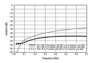
Figure 5. Isolation vs Frequency (ANT to RX, TX to RX, and ANT to TX Ports;  $V_{CTL}=28~V,~I_{CTL}=-50~mA$ )
