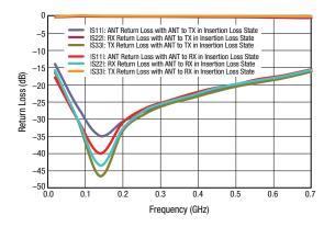
Figure 8. Return Loss vs Frequency (ANT, TX, and RX Ports; VctL = 5 V, IctL = -50 mA)
