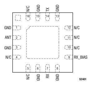
Figure 2. SKY12208-306LF Pinout – 16-Pin QFN (Top View)
