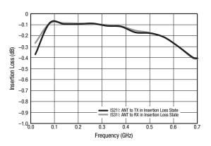
Figure 4. Insertion Loss vs Frequency
