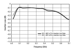
Figure 3. Insertion Loss vs Frequency (ANT to RX and ANT to TX Ports; VctL = 28 V, IctL = -50 mA)
