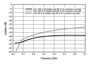
Figure 6. Isolation vs Frequency (ANT to RX, TX to RX, and ANT to TX Ports; VCTL = 5 V, ICTL = -50 mA)
