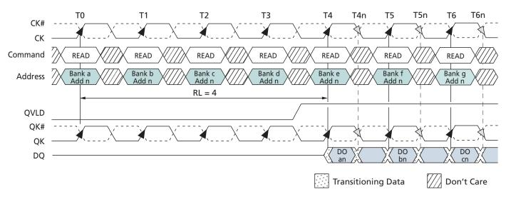
Note: 1. DO an (or bn, cn) = data-out from bank a (or bank b, c) and address n.
