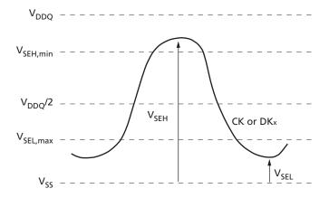
Figure 11: Definition of Differential AC Swing and <sup>t</sup>DVAC
