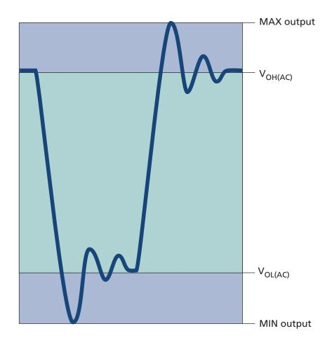
**Figure 17: Differential Output Signal**
