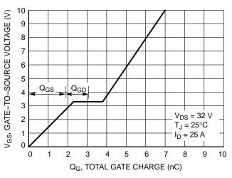
Figure 8. Gate-to-Source vs. Total Charge
