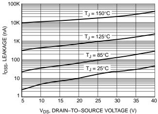
Figure 6. Drain-to-Source Leakage Current vs. Voltage
