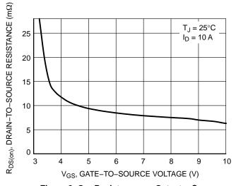
Figure 3. On–Resistance vs. Gate–to–Source Voltage
