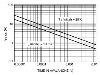
Figure 12. I<sub>PEAK</sub> vs. Time in Avalanche
