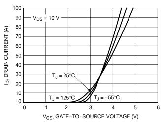
Figure 2. Transfer Characteristics
