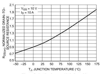
Figure 5. On–Resistance Variation with Temperature
