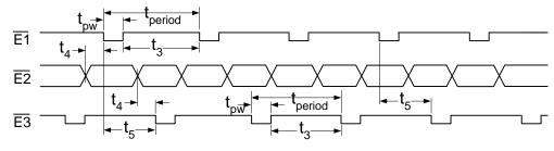
Figure 2. Timing Diagram for  $\overline{E1}$ ,  $\overline{E2}$ , and  $\overline{E3}$
