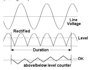
Figure 8. Sag and Fault Detect
