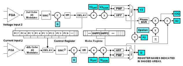
Figure 4. Signal Flow for V2, I2, P2, Q2 Measurements
