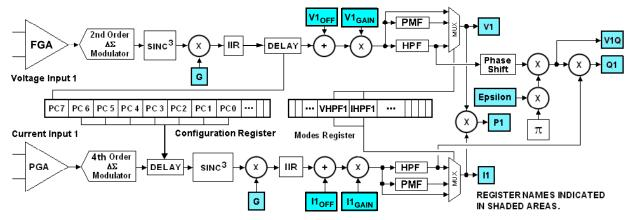
Figure 3. Signal Flow for V1, I1, P1, Q1 Measurements
