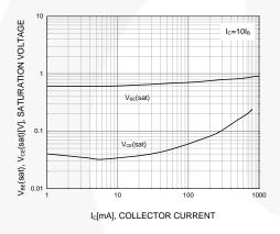
Figure 3. Base-Emitter Saturation Voltage and Collector-Emitter Saturation Voltage
