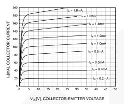
Figure 1. Static Characteristic
