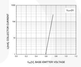
Figure 4. Base-Emitter On Voltage
