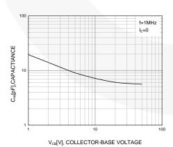
Figure 5. Collector Output Capacitance
