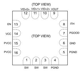
Figure 2. Pin Configuration
