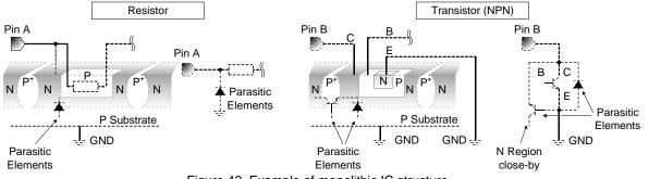
Figure 42. Example of monolithic IC structure
