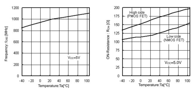
Figure 10. Frequency vs Temperature
