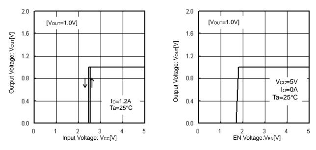
Figure 4. Output Voltage vs Input Voltage
