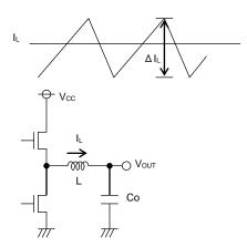
Figure 34. Output ripple current
