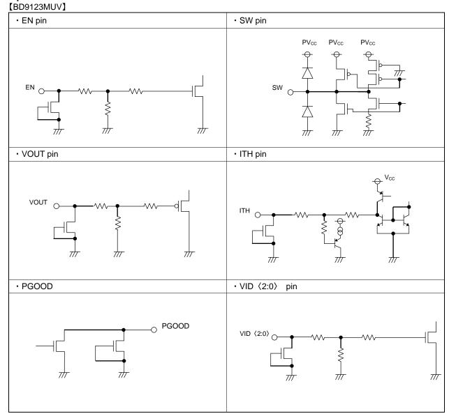
Figure 41. I/O Equivalent Circuit
