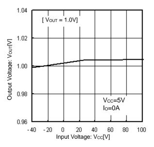
Figure 7. Output Voltage vs Input Voltage
