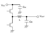
Figure 36. Input Capacitor
