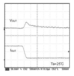
Figure 18. Transient Response (Io=850mA~125mA, 2µA)
