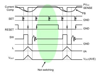
Figure 24. SLLM<sup>™</sup> Switching Timing Chart
