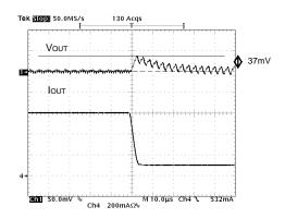
Figure 30. Comparison of Transient Response
