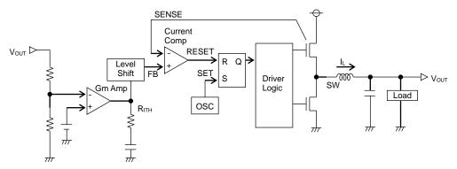
Figure 22. Diagram of Current Mode PWM Control
