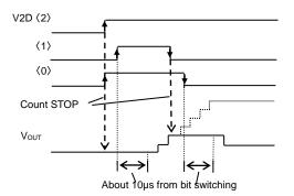
Figure 28. Timing Chart of Setting the Output voltage
