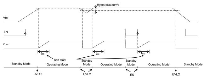
Figure 26. Soft-Start, Shutdown, UVLO Timing Chart
