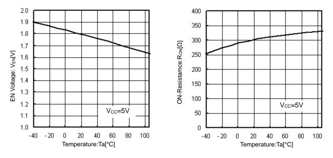
Figure 12. EN Voltage vs Temperature
