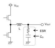
Figure 35. Output Capacitor
