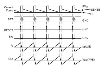
Figure 23. PWM Switching Timing Chart
