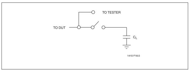
Figure 20: A Test Load Example
