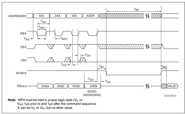
Figure 6: WE# Controlled Program Cycle Timing Diagram
