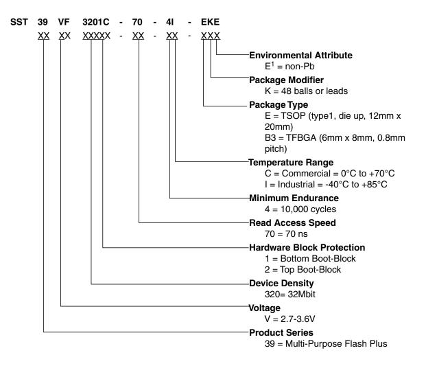
1. Environmental suffix "E" denotes non-Pb solder. non-Pb solder devices are "RoHS Compliant".
