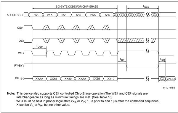
Figure 10:WE# Controlled Chip-Erase Timing Diagram
