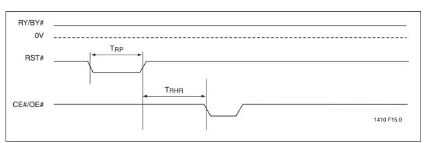
Figure 17:RST# Timing Diagram (When no internal operation is in progress)
