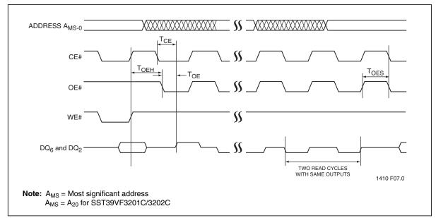
Figure 9: Toggle Bits Timing Diagram
