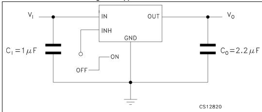
Note: Inhibit pin is not internally pulled-up then it must not be left floating. Disable the device when connected to GND or to a positive voltage less than 0.18 V.
