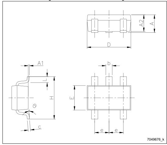
Figure 23. SOT23-5L mechanical drawing
