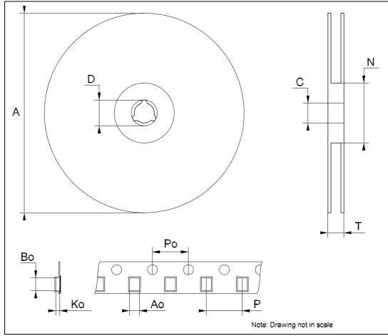
Figure 25. Tape and reel SOT23-5L mechanical drawing
