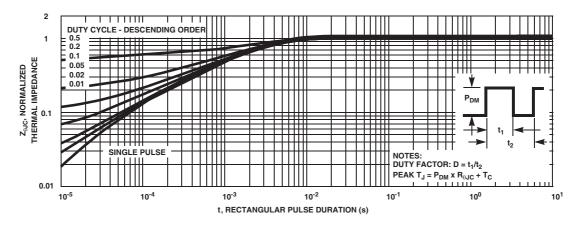
Figure 3. Normalized Maximum Transient Thermal Impedance
