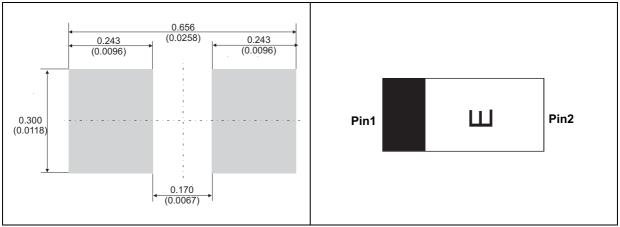
Note: The marking codes can be rotated by 90° or 180° to differentiate assembly location. In no case should this product marking be used to orient the component for its placement on a PCB. Only pin 1 mark is to be used for this purpose.
