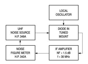
Figure 5. Noise Figure Test Circuit
