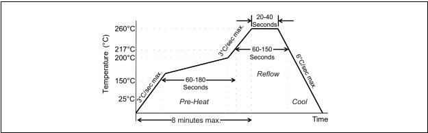
FIGURE 5-1: Solder Reflow Profile.
