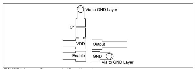
FIGURE 3-3: Recommended Board Layout.
