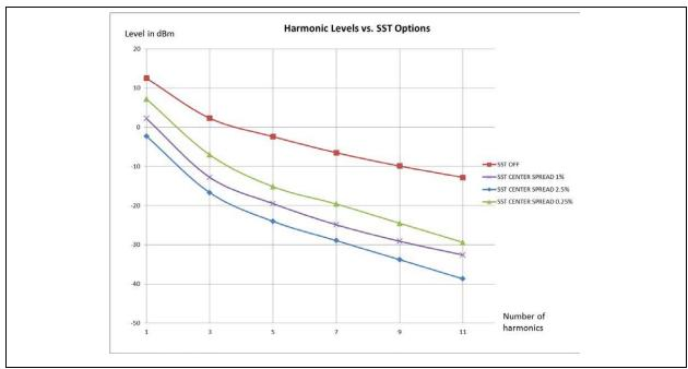
FIGURE 4-3: DSC6331 Harmonic Levels with Various Spread Spectrum Options.
