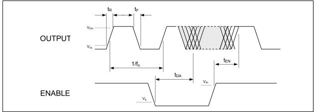
FIGURE 3-1: Output Waveform.
