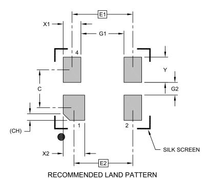
Units MILLIMETERS **Dimension Limits** MIN NOM MAX Contact Pitch E1 1.20 BSC Contact Pitch E2 1.16 BSC Contact Spacing С 0.75 0.35 Contact Width (X3) X1 Contact Width X2 0.43 Contact Pad Length (X6) Υ 0.50 Space Between Contacts (X4) G1 0.85 Space Between Contacts (X3) G2 0.25 0.13 X 45° REF Contact 1 Index Chamfer СН
