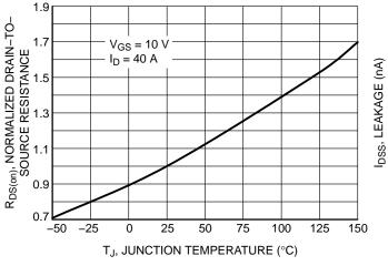
Figure 5. On–Resistance Variation with Temperature
