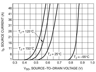
Figure 10. Diode Forward Voltage vs. Current
