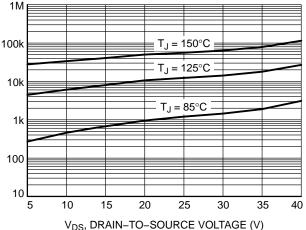
Figure 6. Drain-to-Source Leakage Current vs. Voltage
