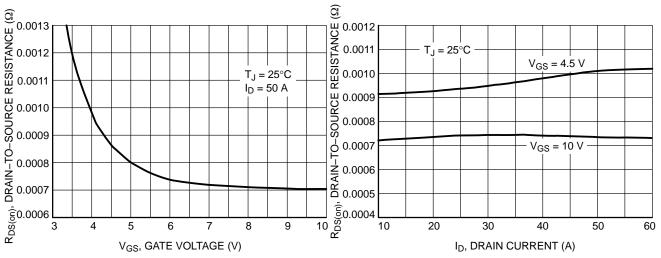
Figure 3. On–Resistance vs. Gate–to–Source Voltage
