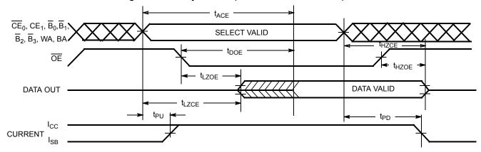
Figure 6. Read Cycle No. 3 (Either Port)  $^{[35,\ 37,\ 38,\ 39]}$
