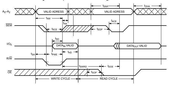
Figure 10. Timing Diagram of Semaphore Contention [50, 51, 52]
