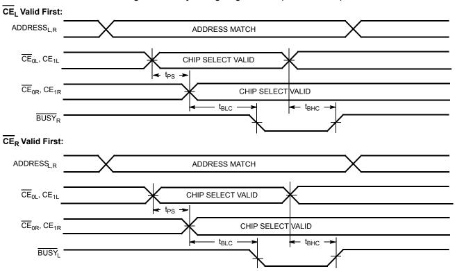
Figure 14. Busy Timing Diagram No. 2 (Address Arbitration)  $^{[54]}$
