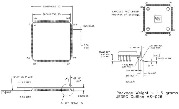
(DIMENSIONS ARE IN MILLIMETERS)
