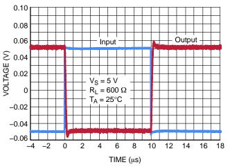
Figure 18. Inverting Small Signal Transient Response
