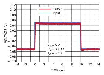
Figure 17. Noninverting Small Signal Transient Response
