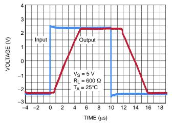
Figure 19. Noninverting Large Signal Transient Response
