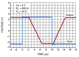
Figure 20. Inverting Large Signal Transient Response
