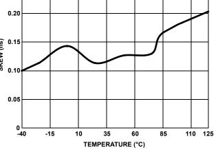
FIGURE 15. DRIVER DIFFERENTIAL SKEW vs TEMPERATURE
