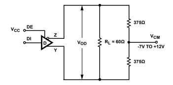
FIGURE 4A.  $V_{OD}$  AND  $V_{OC}$
