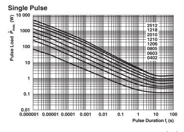
Maximum pulse load, single pulse; applicable if  $\bar{P} \to 0$  and n < 1000 and  $\hat{U} \le \hat{U}_{max}$ ; for permissible resistance change equivalent to 8000 h operation
