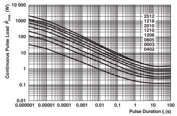
Maximum pulse load, continuous pulses; applicable if  $\bar{P} \leq P \; (\vartheta_{amb})$  and  $\hat{U} \leq \hat{U}_{max}$ ; for permissible resistance change equivalent to 8000 h operation
