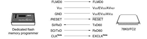
Note The above figure illustrates an example of wiring when using the clock output from the PG-FP4 or FL-PR4. When using the clock output from the PG-FPL3 or FP-LITE3, connect CLK to X1/P121 (pin 8;  $\mu$ PD78F0881, 78F0882, 78F0883, pin 9;  $\mu$ PD78F0884, 78F0885, 78F0886), and connect its inverted signal to X2/EXCLK/P122 (pin 7;  $\mu$ PD78F0881, 78F0882, 78F0883, pin 8;  $\mu$ PD78F0884, 78F0885, 78F0886).
