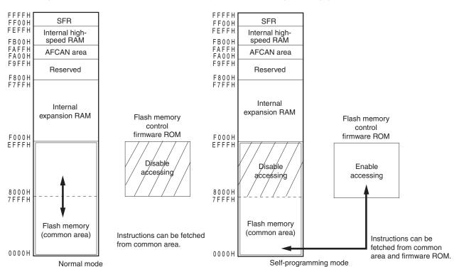
Figure 23-17. Operation Mode and Memory Map for Self-Programming (μPD78F0883, 78F0886)
