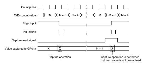
Figure 6-45. Timing of Holding Data by Capture Register
