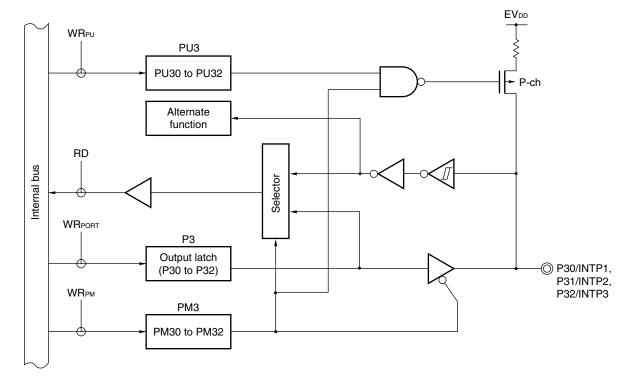
Figure 4-8. Block Diagram of P30 to P32
