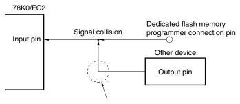
In the flash memory programming mode, the signal output by the device collides with the signal sent from the dedicated flash memory programmer. Therefore, isolate the signal of the other device.
