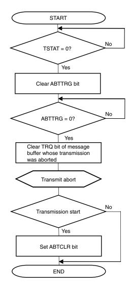
Figure 15-49. ABT Transmission Abort Processing (Normal Operation Mode with ABT)
