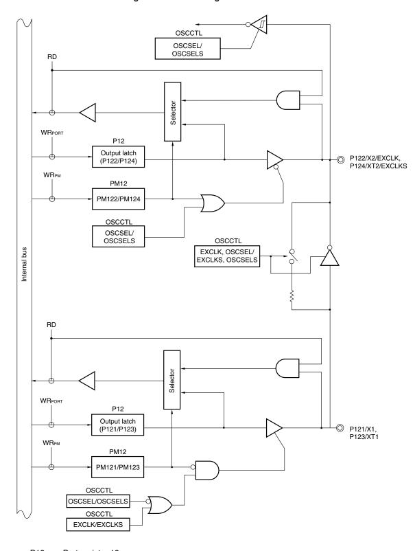
Figure 4-18. Block Diagram of P121 to P124
