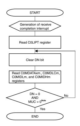
Figure 15-51. Reception via Interrupt (Using C0LIPT Register)
