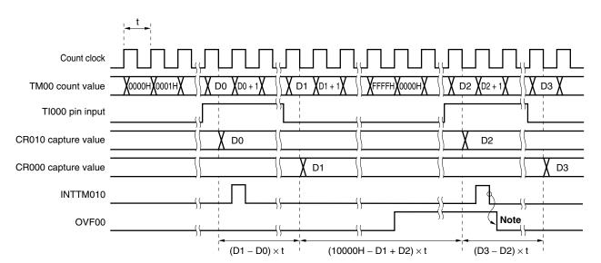
Figure 6-30. Timing of Pulse Width Measurement Operation with Free-Running Counter and Two Capture Registers (with Rising Edge Specified)
