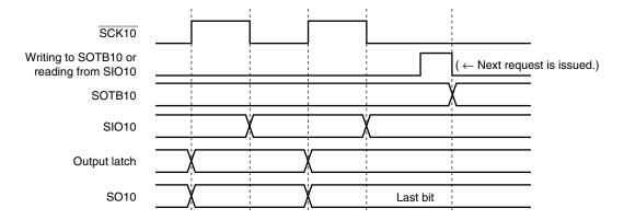
Figure 14-8. Output Value of SO10 Pin (Last Bit) (2/2)
