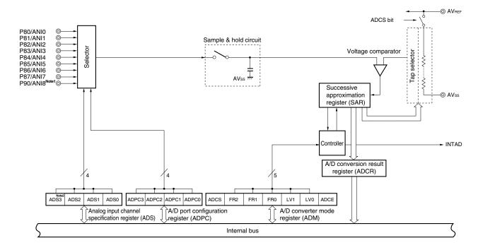
Figure 12-1. Block Diagram of A/D Converter
