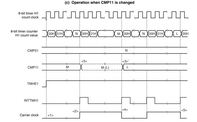
Figure 8-15. Carrier Generator Mode Operation Timing (3/3)
