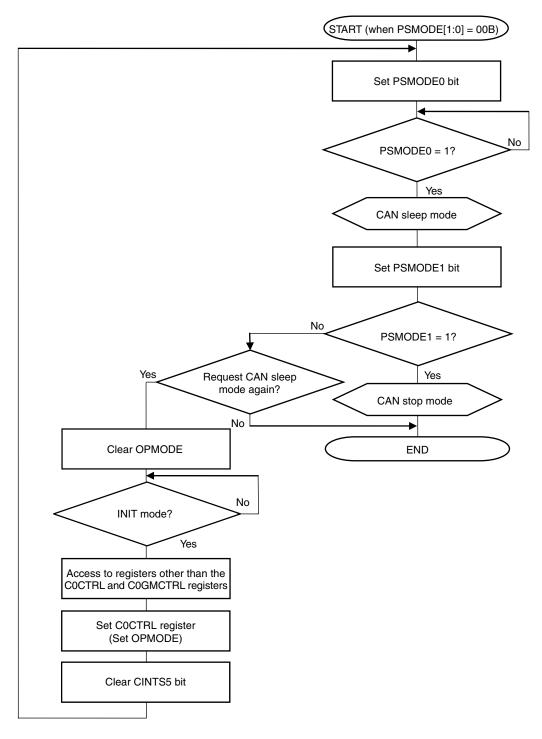
Figure 15-54. Setting CAN Sleep Mode/Stop Mode
