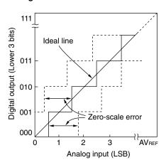
Figure 12-19. Integral Linearity Error
