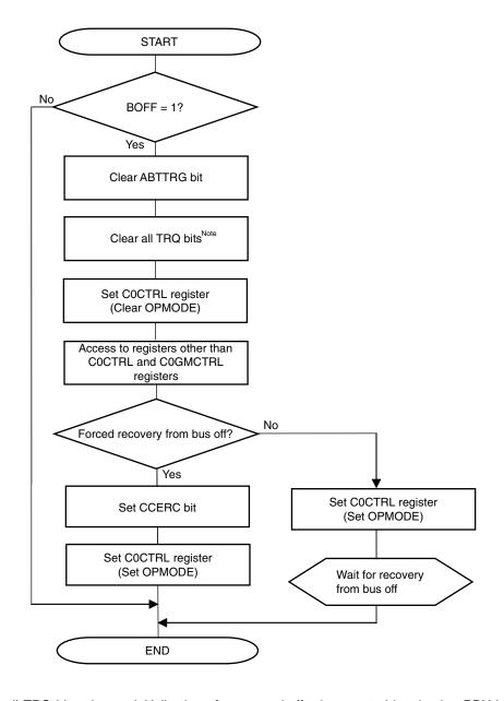
Figure 15-57. Bus-Off Recovery (Normal Operation Mode with ABT)
