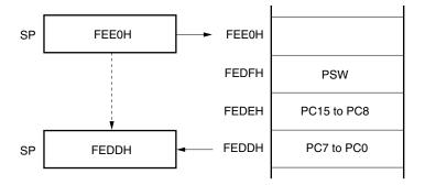
Figure 3-11. Data to Be Restored from Stack Memory
