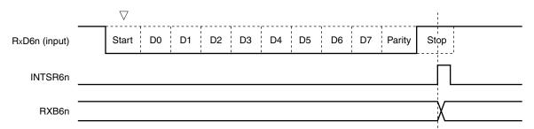
Figure 13-27. Reception Completion Interrupt Request Timing
