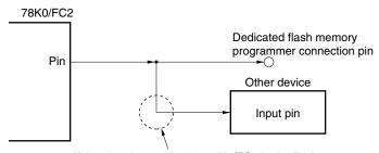
If the signal output by the 78K0/FC2 in the flash memory programming mode affects the other device, isolate the signal of the other device.
