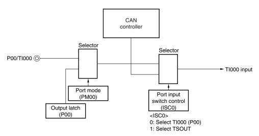
Figure 15-36. Port Input Switch Control
