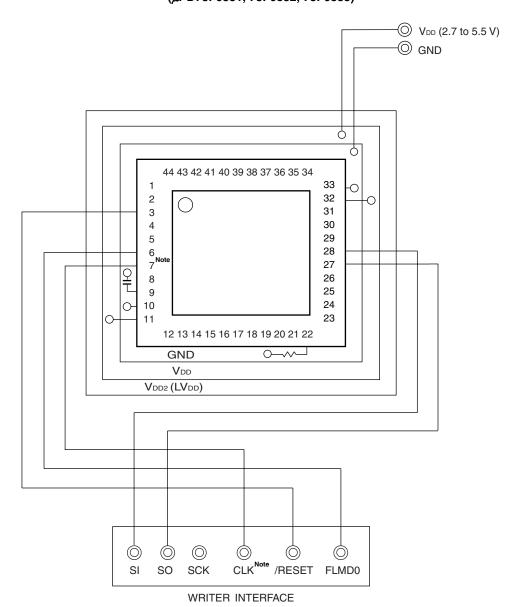
Figure 23-4. Example of Wiring Adapter for Flash Memory Writing in UART (UART60) Mode  $(\mu PD78F0881, 78F0882, 78F0883)$
