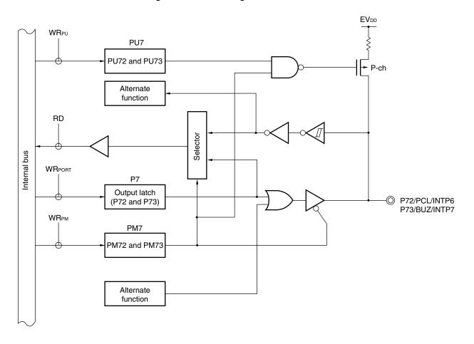
Figure 4-14. Block Diagram of P72 and P73
