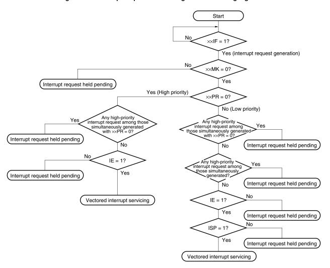
Figure 16-7. Interrupt Request Acknowledgement Processing Algorithm
