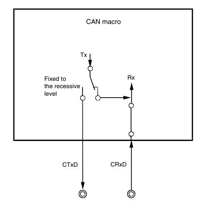
Figure 15-33. CAN Module Terminal Connection in Receive-Only Mode
