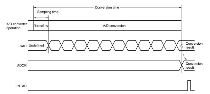
Figure 12-12. Basic Operation of A/D Converter
