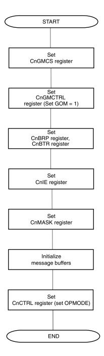
**Remark** OPMODE: Normal operation mode, normal operation mode with ABT, receive-only mode, single-shot mode, self-test mode
