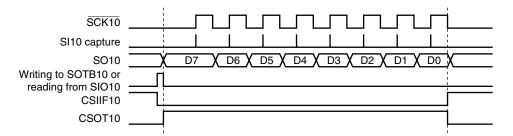
**Remark** The above figure illustrates a communication operation where data is transmitted with the MSB first.
