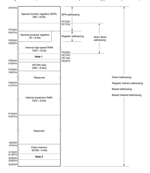
Figure 3-4. Correspondence Between Data Memory and Addressing (µPD78F0881, µPD78F0884)
