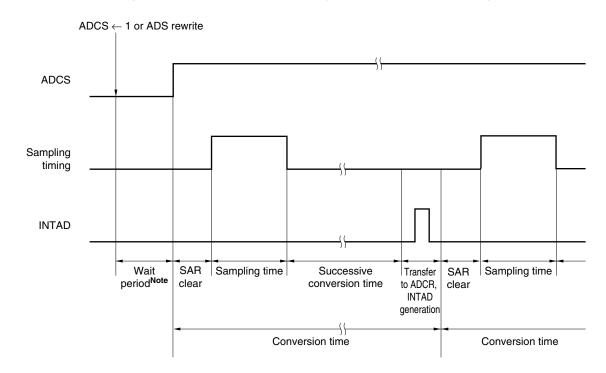
Figure 12-5. A/D Converter Sampling and A/D Conversion Timing
