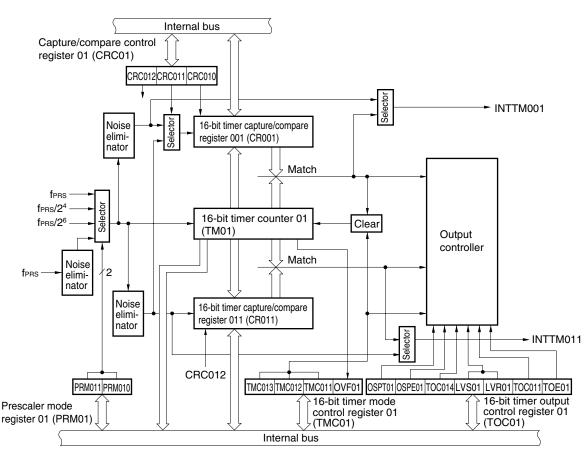
Figure 6-2. Block Diagram of 16-Bit Timer/Event Counter 01 (μPD78F0881, 78F0882, 78F0883)
