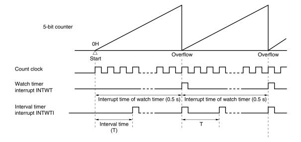
Figure 9-3. Operation Timing of Watch Timer/Interval Timer
