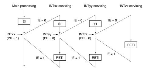
During servicing of interrupt INTxx, two interrupt requests, INTyy and INTzz, are acknowledged, and multiple interrupt servicing takes place. Before each interrupt request is acknowledged, the El instruction must always be issued to enable interrupt request acknowledgment.
