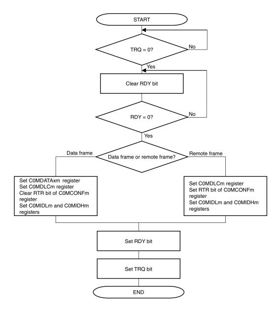
Figure 15-42. Message Transmit Processing
