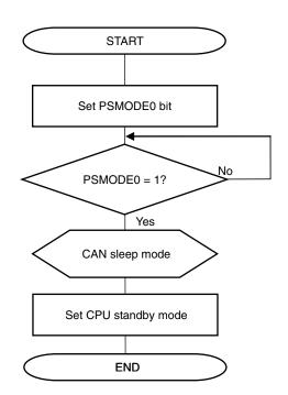
Figure 15-61. Setting CPU Standby (from CAN Sleep Mode)
