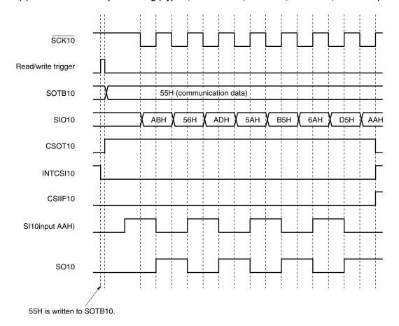
Figure 14-6. Timing of Clock/Data Phase
