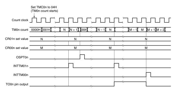
Figure 6-39. Timing of One-Shot Pulse Output Operation with Software Trigger
