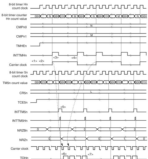
Figure 8-15. Carrier Generator Mode Operation Timing (2/3)
