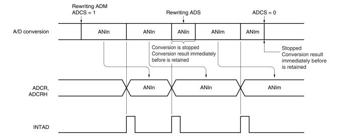
Figure 12-14. A/D Conversion Operation
