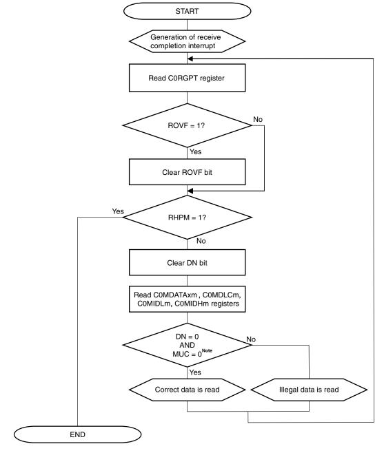
Figure 15-52. Reception via Interrupt (Using C0RGPT Register)
