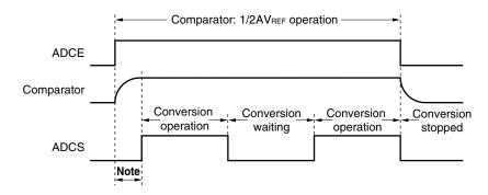
**Note** To stabilize the internal circuit, the time from the rising of the ADCE bit to the rising of the ADCS bit must be 1  $\mu$ s or longer.
