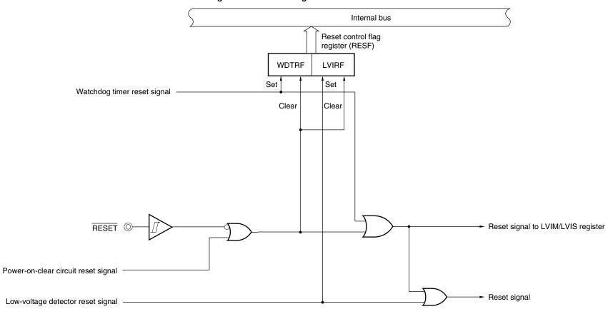
Figure 18-1. Block Diagram of Reset Function
