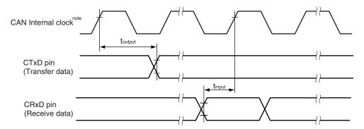
Internal delay time (tnode) = Internal Transfer Delay (toutput) + Internal Receive Delay (tinput)
