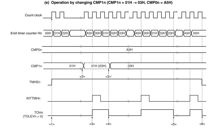
Figure 8-12. Operation Timing in PWM Output Mode (4/4)
