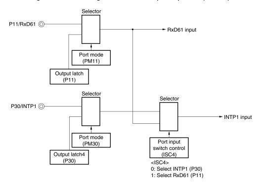
Figure 13-4. Port Configuration for LIN Reception Operation (UART61)
