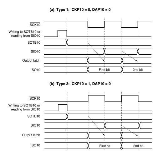
Figure 14-7. Output Operation of First Bit (1/2)
