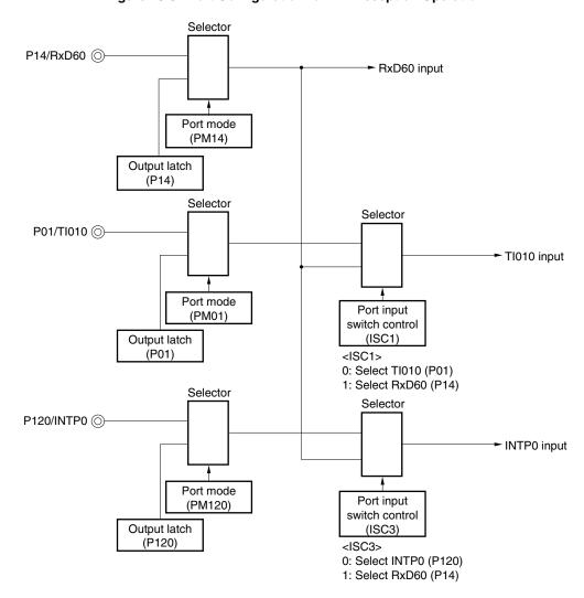
Figure 13-3. Port Configuration for LIN Reception Operation
