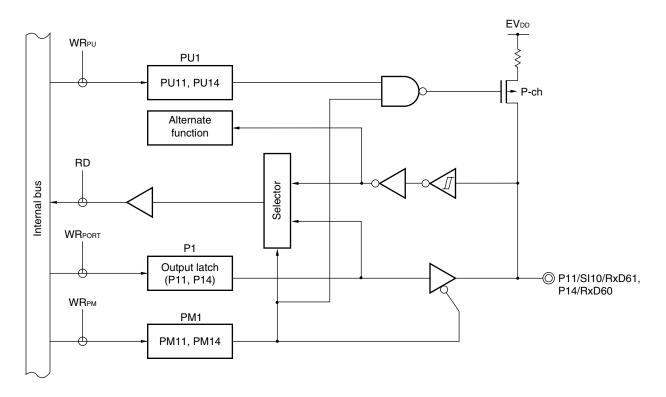
Figure 4-6. Block Diagram of P11 and P14
