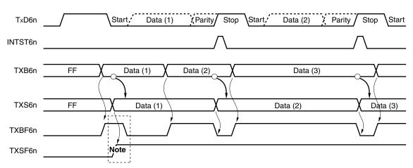
Figure 13-25. Timing of Starting Continuous Transmission
