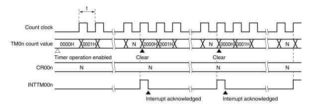
Figure 6-19. Timing of Interval Timer Operation
