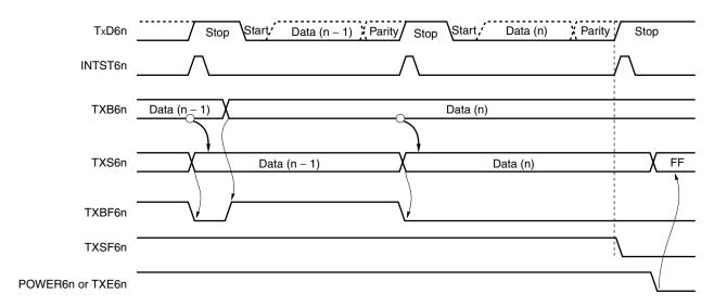
Figure 13-26. Timing of Ending Continuous Transmission
