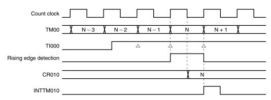
Figure 6-23. CR010 Capture Operation with Rising Edge Specified
