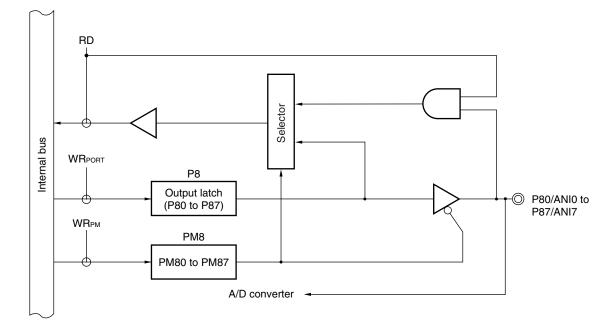
Figure 4-15. Block Diagram of P80 to P87
