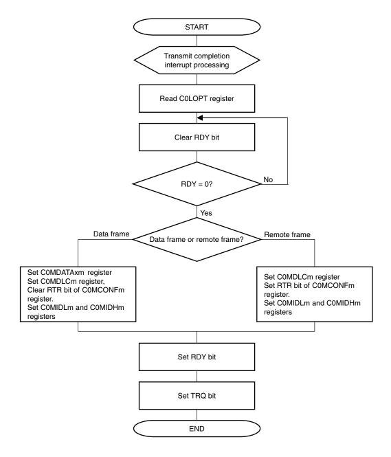
Figure 15-44. Transmission via Interrupt (Using C0LOPT register)
