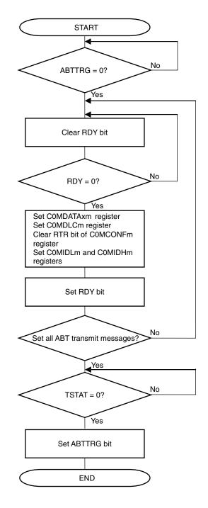
Figure 15-43. ABT Message Transmit Processing
