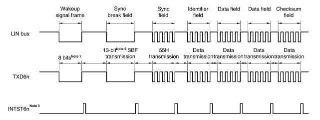
Figure 13-1. LIN Transmission Operation
