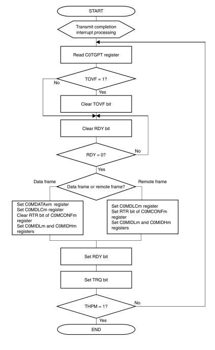
Figure 15-45. Transmit via Interrupt (Using C0TGPT register)
