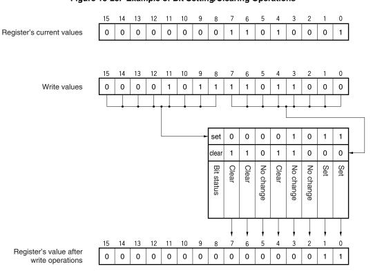
Figure 15-24. 16-Bit Data during Write Operation
