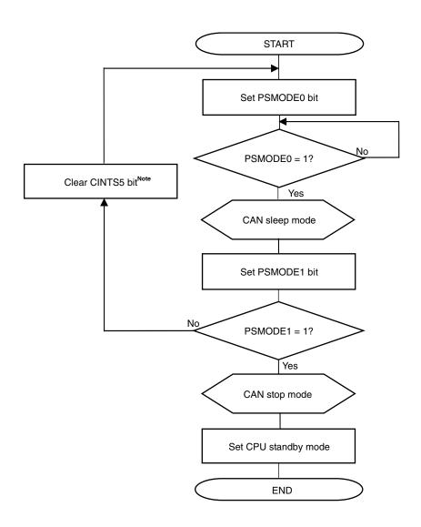
Figure 15-62. Setting CPU Standby (from CAN Stop Mode)
