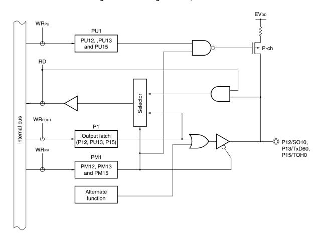
Figure 4-7. Block Diagram of P12, P13 and P15
