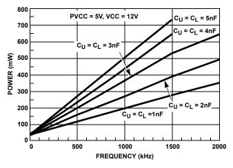
FIGURE 6. POWER DISSIPATION vs FREQUENCY, PVCC = 5V
