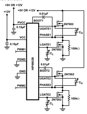
FIGURE 1. HIP6602B TEST CIRCUIT
