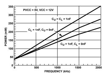
FIGURE 7. POWER DISSIPATION vs FREQUENCY, PVCC = 5V
