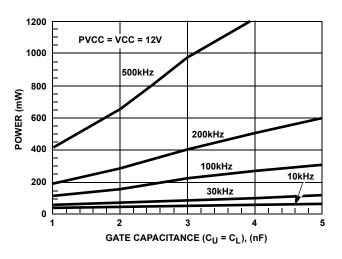
FIGURE 5. POWER DISSIPATION vs LOADING
