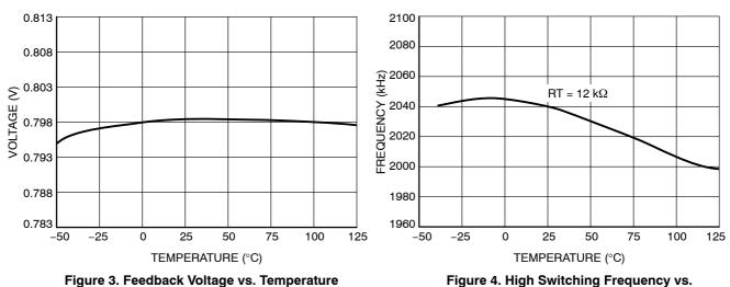
Figure 3. Feedback Voltage vs. Temperature
