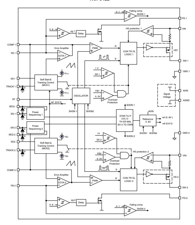
Figure 2. Block Diagram
