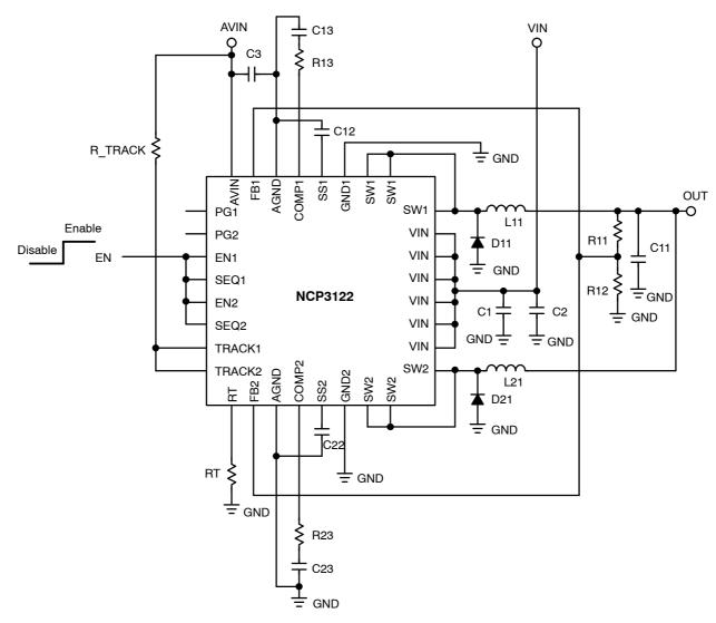
Figure 73. Parallel Operation Configuration.
