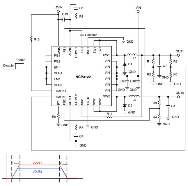
Figure 54. Tracking Configuration
