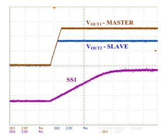
Figure 56. Tracking Mode - Power-up
