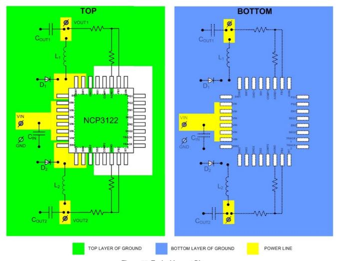
Figure 75. Typical Layout Diagram
