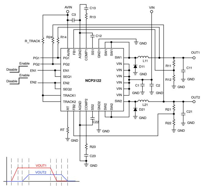
Figure 71. Normal Operation Configuration
