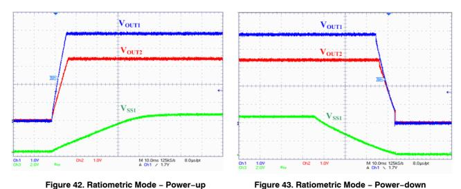
Figure 42. Ratiometric Mode - Power-up
