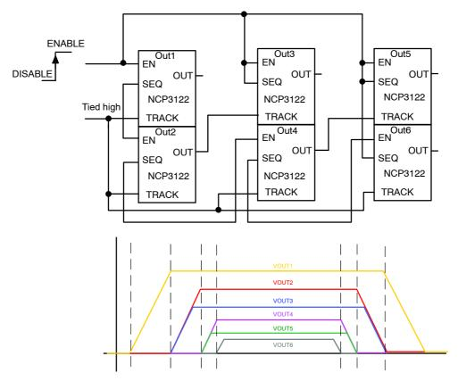
Figure 68. Mixed Mode, Configuration B
