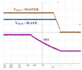
Figure 57. Tracking Mode - Power-down
