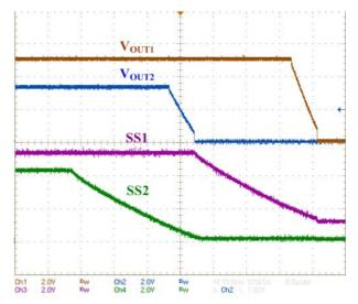
Figure 50. Sequential Mode - Power-down
