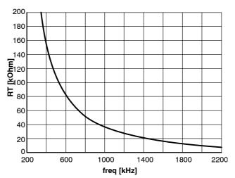
Figure 39. Switching Frequency Selection
