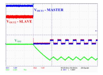
Figure 61. Master Voltage - Start of OLM
