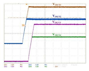
Figure 66. Mixed Mode of Four Outputs – Power-up
