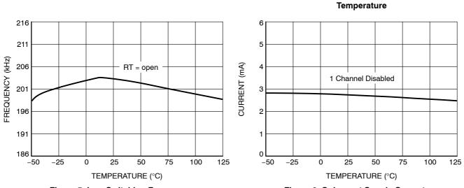
Figure 5. Low Switching Frequency vs. Temperature
