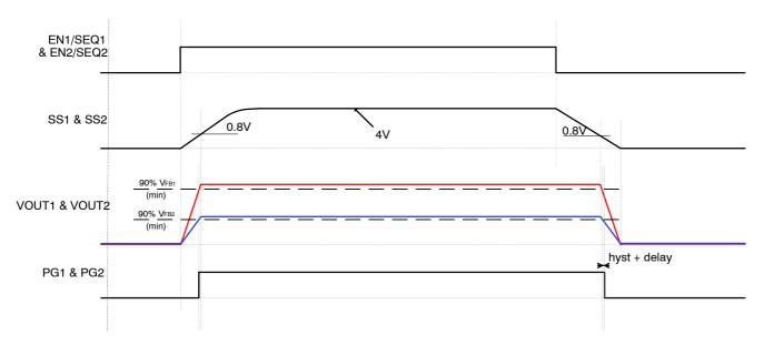
Figure 41. Typical Behavior of Ratiometric Sequencing Mode
