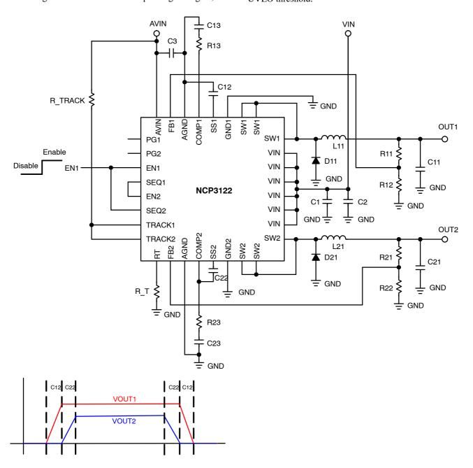
Figure 46. Sequential Configuration
