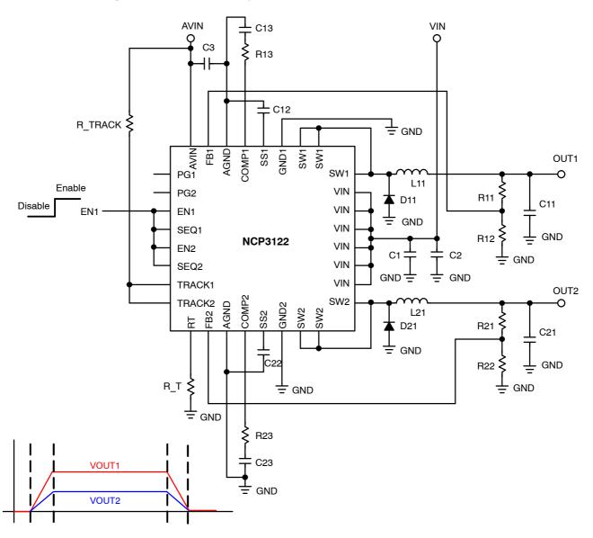
Figure 40. Ratiometric Sequencing Configuration
