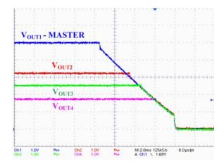
Figure 59. Tracking Mode of Four Outputs –
