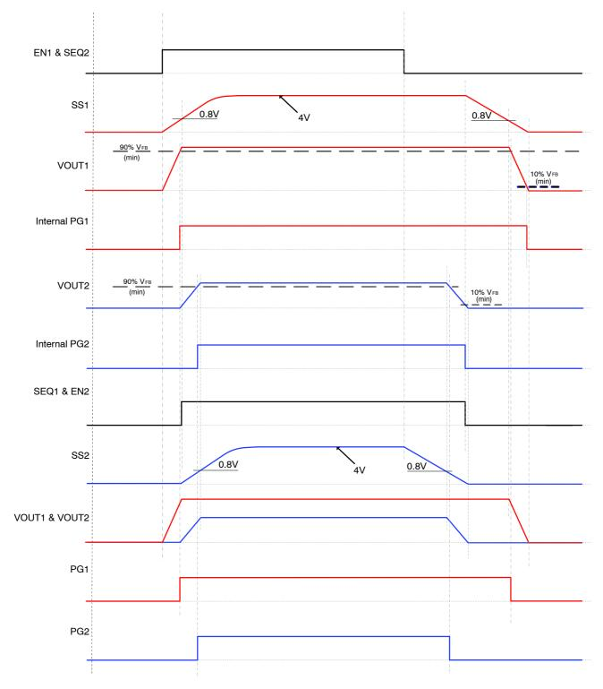
Figure 48. Typical Behavior of Sequential Mode
