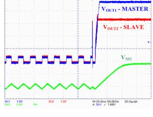
Figure 62. Master Voltage - End of OLM
