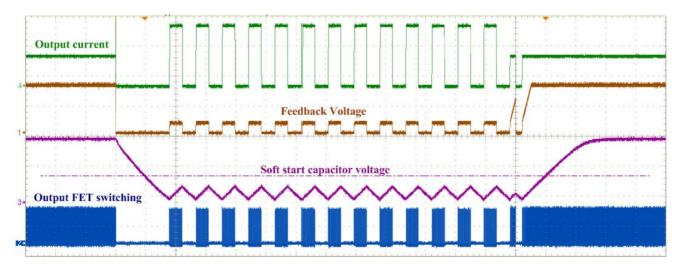
Figure 37. Hiccup Overload Protection
