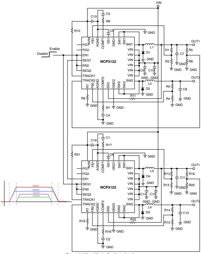
Figure 65. Mixed Mode, Configuration A
