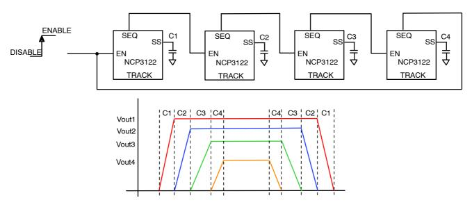
Figure 47. Simplified Drawing of Daisy-chained NCP3122's
