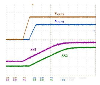
Figure 49. Sequential Mode - Power-up
