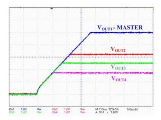
Figure 58. Tracking Mode of Four Outputs – Power-up
