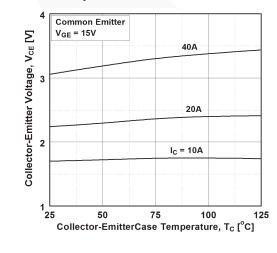
Figure 2. Typical Output Characteristics
