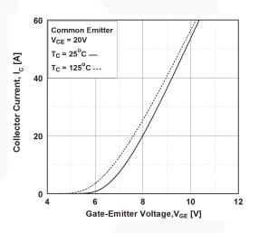
Figure 6. Saturation Voltage vs. V<sub>GE</sub>
