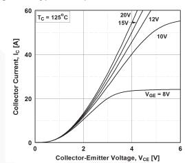
**Figure 4. Transfer Characteristics**
