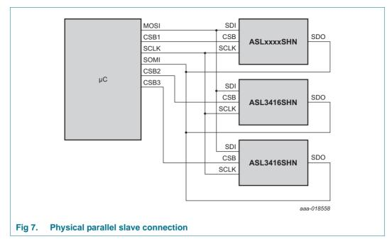
During the SPI data transfer, the identifier byte and the actual content of the addressed registers is returned via the SDO pin. The same happens for pure read accesses. Here the read-only bit must be set to 1. The content of the data bytes that are transmitted to the ASL3416SHN is ignored.
