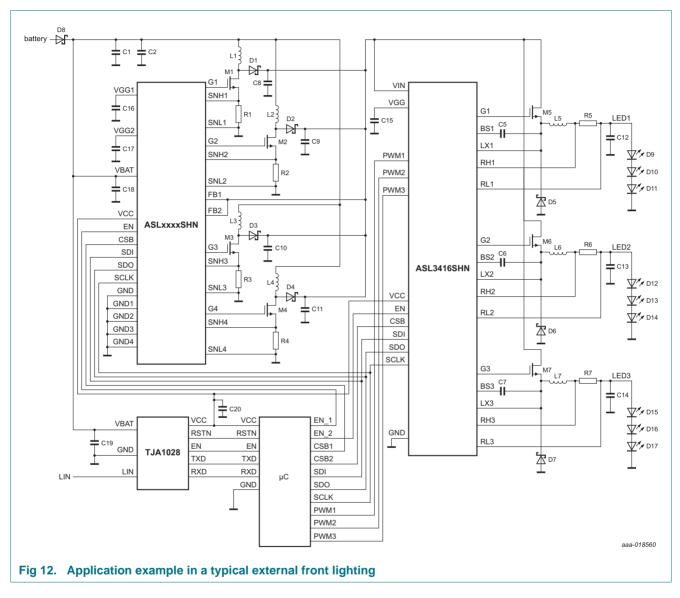
Figure 12 provides an example for the ASL3416SHN in a typical external front lighting application driving 3 independent LED strings.
