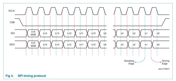
The data bits of the ASL3416SHN are arranged in registers of 1 byte length. Each register is assigned to a 7-bit address. For writing into a register, 2 bytes must be sent to the LED driver. The first byte is an identifier byte that consists of the 7-bit address and one read-only bit. For writing, the read-only bit must be set to "0". The second byte is the data that shall be written into the register. So an SPI access consists of at least 16 bits.
